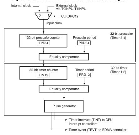
Figure 4. Dual 32-Bit Timers Chained Mode Block Diagram
