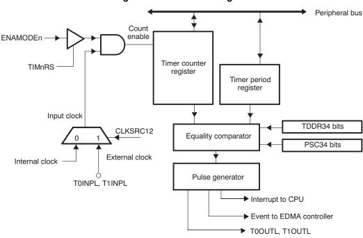
Figure 1. Timer Block Diagram
