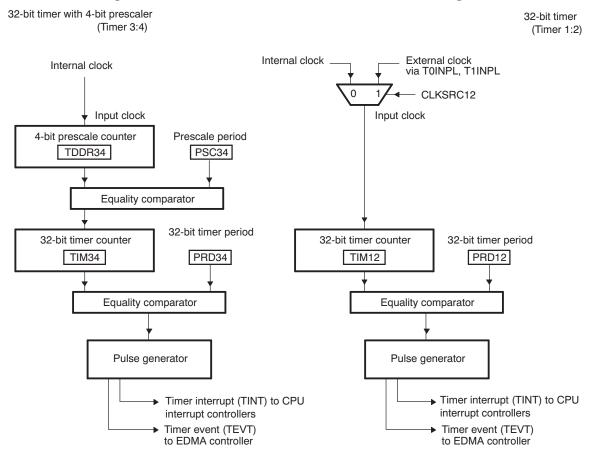
Figure 6. Dual 32-Bit Timers Unchained Mode Block Diagram
