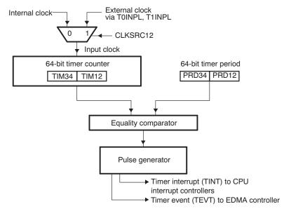
Figure 3. 64-Bit Timer Mode Block Diagram
