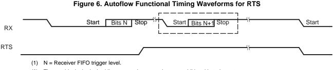
(2) The two blocks in dashed lines cover the case where an additional byte is sent.
