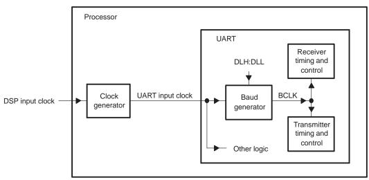
Figure 2. UART Clock Generation Diagram
