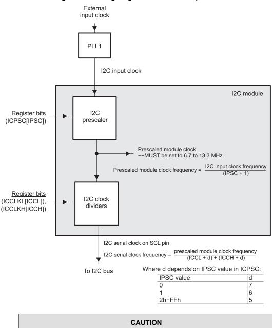
Figure 3. Clocking Diagram for the I2C Peripheral
