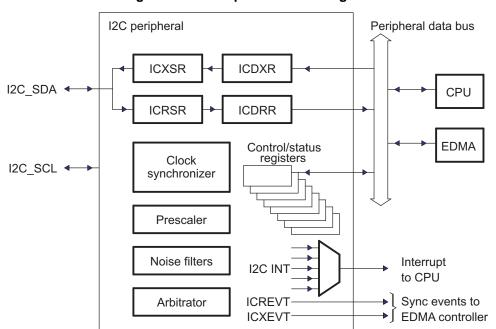
Figure 1. I2C Peripheral Block Diagram
