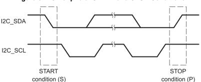
Figure 6. I2C Peripheral START and STOP Conditions
