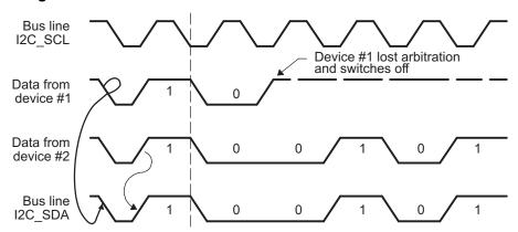
Figure 12. Arbitration Procedure Between Two Master-Transmitters
