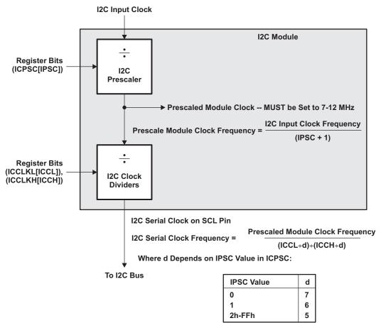
Figure 3. Clocking Diagram for the I2C Peripheral
