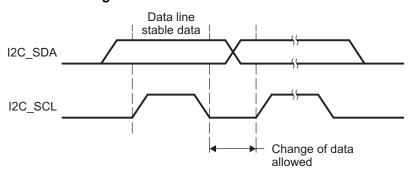
Figure 5. Bit Transfer on the I2C-Bus
