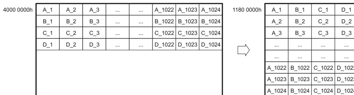
**Figure 20. Data Sorting Example PaRAM Configuration**
