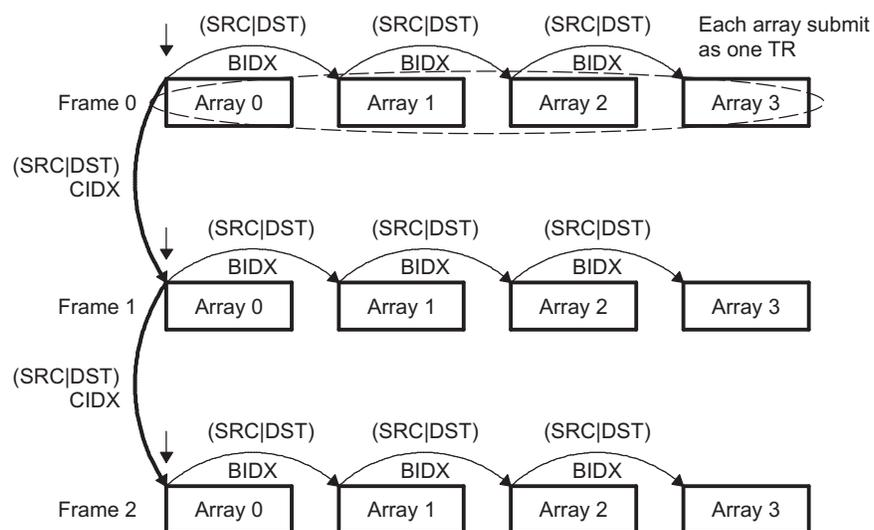
**NOTE:** ABC-synchronized transfers are not directly supported. But can be logically achieved by chaining between multiple AB-synchronized transfers.
