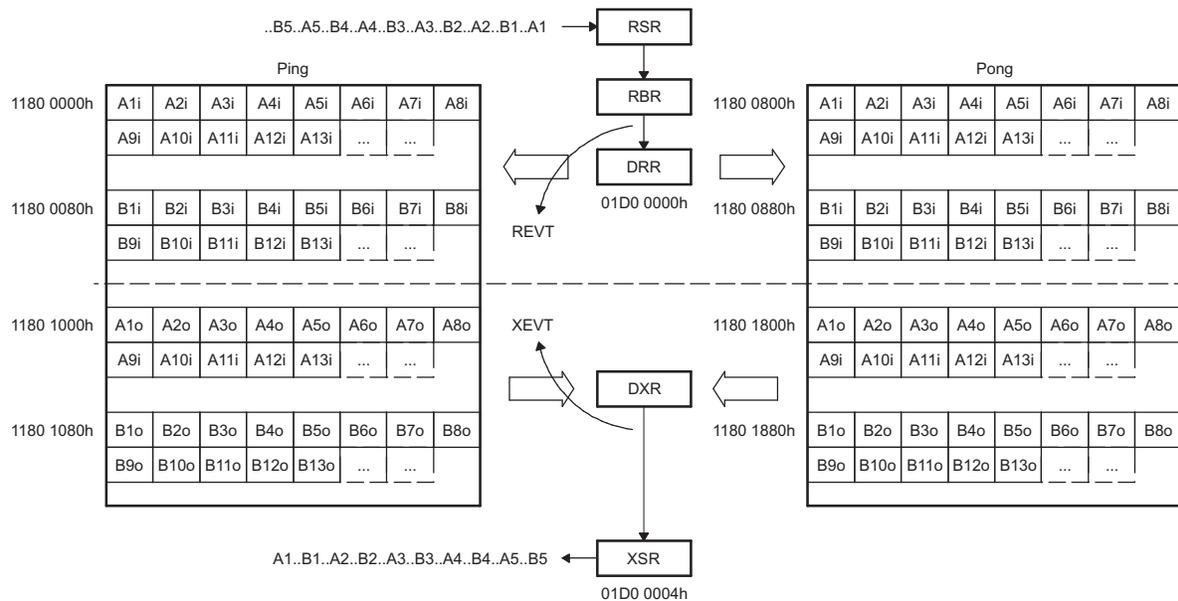
**Figure 29. Ping-Pong Buffering for McBSP Example PaRAM**
