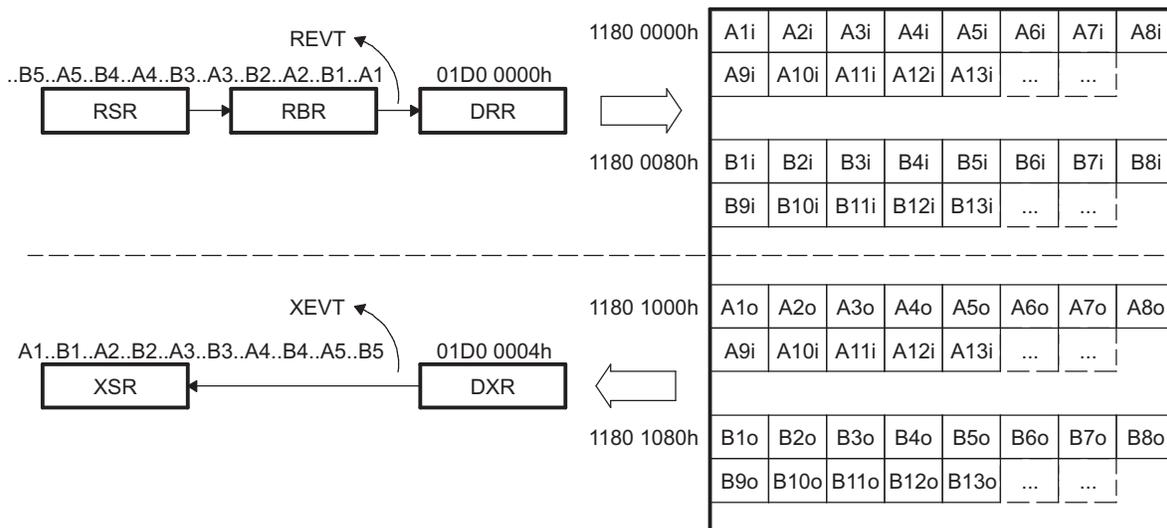
**Figure 26. Servicing Continuous McBSP Data Example PaRAM**
