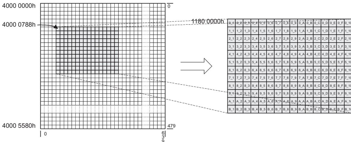
Figure 18. Subframe Extraction Example PaPARAM Configuration
