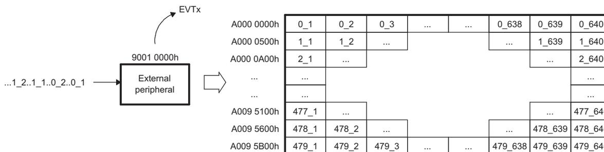
Figure 24. Servicing Peripheral Burst Example PaRAM
