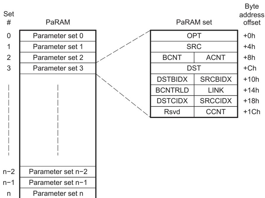
Note:  $n$  is the number of PaRAM sets supported in the EDMA3CC for a specific device.
