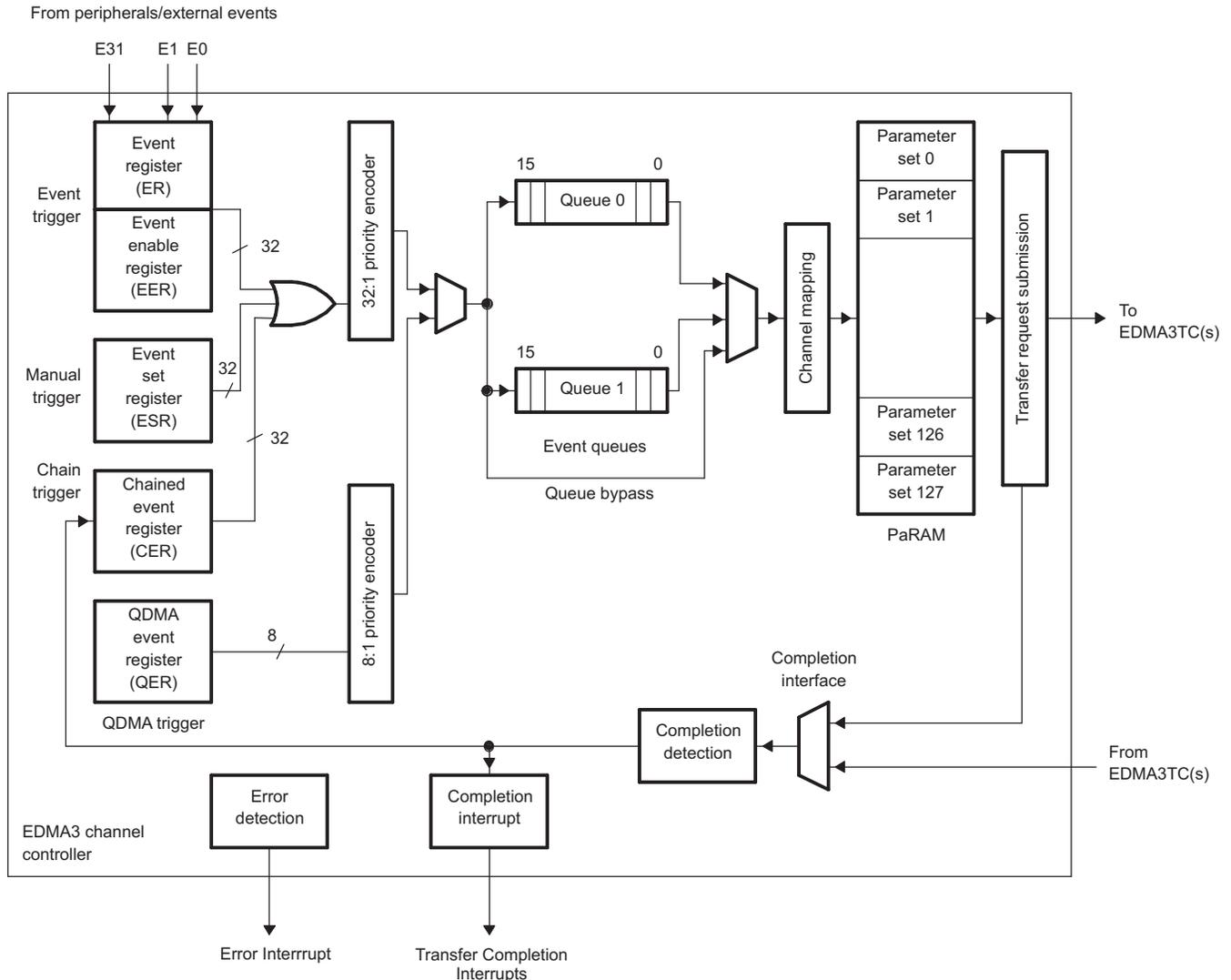
Each event in the event queue is processed in the order it was queued. On reaching the head of the queue, the PaRAM associated with that channel is read to determine the transfer details. The TR submission logic evaluates the validity of the TR and is responsible for submitting a valid transfer request (TR) to the appropriate EDMA3TC (based on the event queue to EDMA3TC association, Q0 goes to TC0, and Q1 goes to TC1, etc.). For more details, see [Section 2.3](#).
