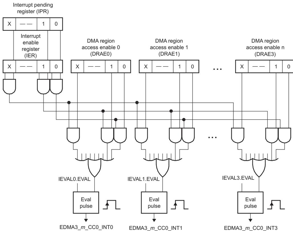
**NOTE:** The DRAE for all regions is expected to be set up at system initialization and to remain static for an extended period of time. The interrupt enable registers should be used for dynamic enable/disable of individual interrupts.
