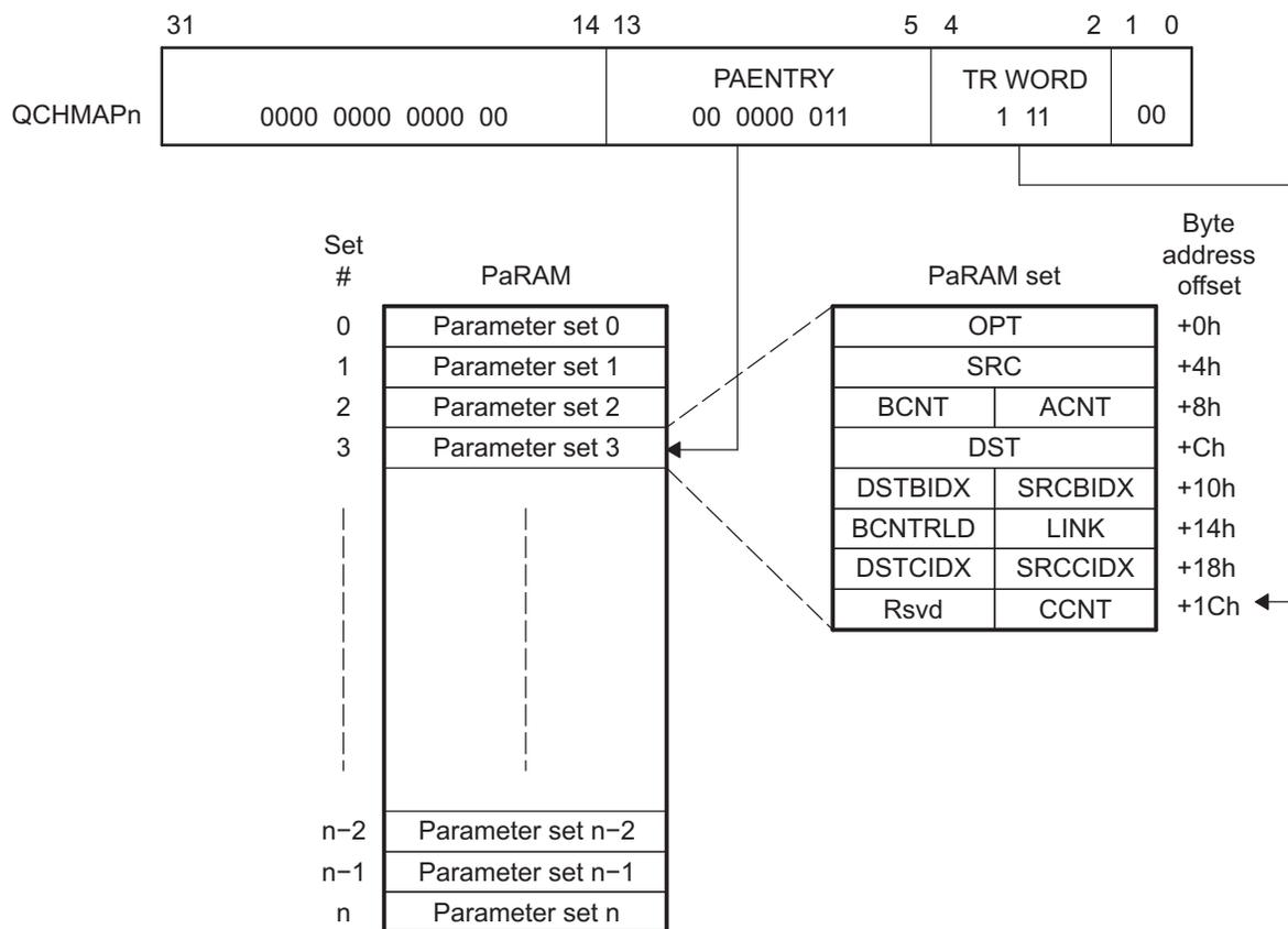
Note:  $n$  is the number of PaRAM sets supported in the EDMA3CC for a specific device.
