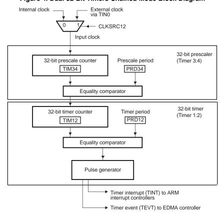
Figure 4. Dual 32-Bit Timers Chained Mode Block Diagram
