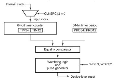
Figure 9. Watchdog Timer Mode Block Diagram
