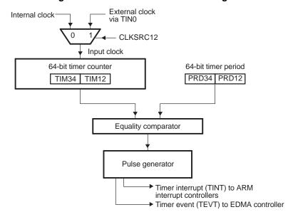
Figure 3. 64-Bit Timer Mode Block Diagram
