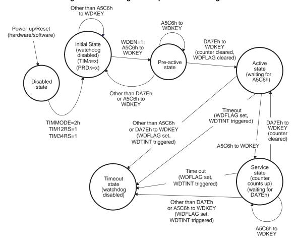
Figure 10. Watchdog Timer Operation State Diagram
