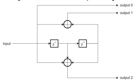
Figure 1. Convolutional Encoder Example Block Diagram
