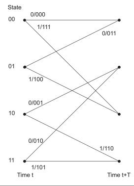
**NOTE:** K = 3, R = k/n = 1/3,  $G_0 = (100)_8$ ,  $G_1 = (101)_8$ ,  $G_2 = (111)_8$  0/000 means input is 0, output1 is 0, output2 is 0, output3 is 0. There are  $2^{(K-1)}$  states and  $2^k$  incoming branches per state.
