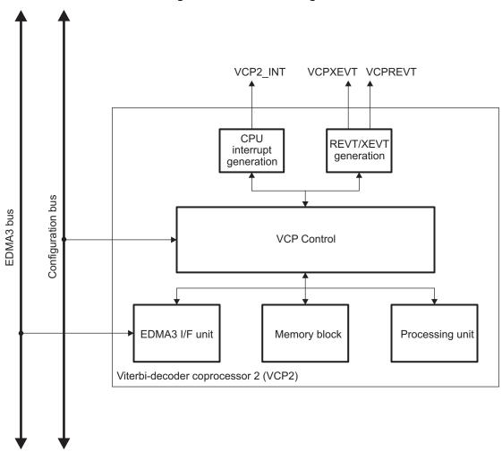
Figure 3. VCP2 Block Diagram
