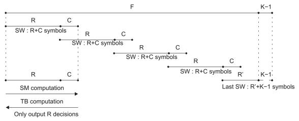
Figure 27. Convergent Traceback Mode-Example With Five Sliding Windows
