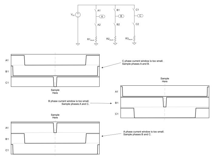
Figure 5. Inverter Using the 3-Shunt Current Sampling Technique
