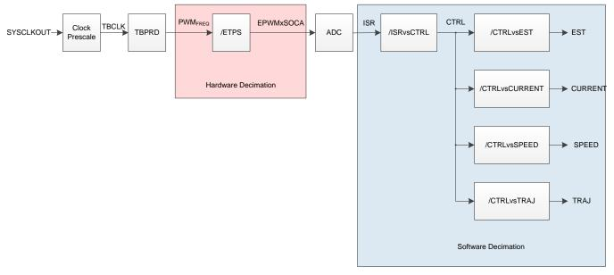
Figure 6. Software Execution Clock Tree Provides Flexibility with Real-Time Scheduling
