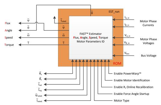
Figure 1. FAST - Estimating Flux, Angle, Speed, Torque - Automatic Motor Identification
