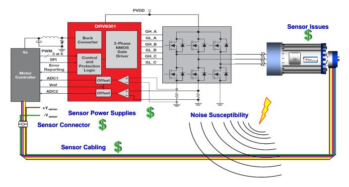
Figure 4. Sensored FOC System
