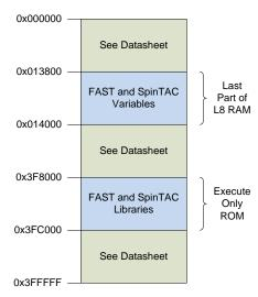
Figure 8. 2806xF Allocated Memory for InstaSPIN-FOC Library
