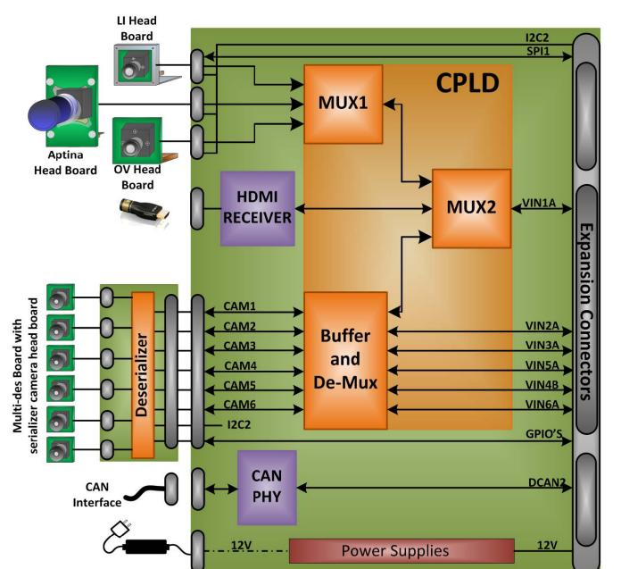
Figure 1 shows the block diagram of the vision application board.
