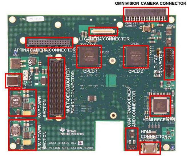
Figure 4. Board With Components Identifications
