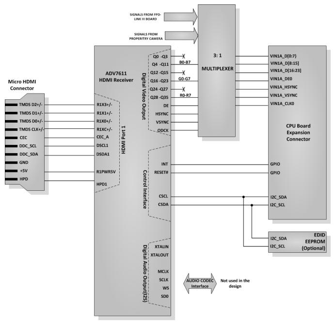
Figure 12. HDMI Signal-Level Connections
