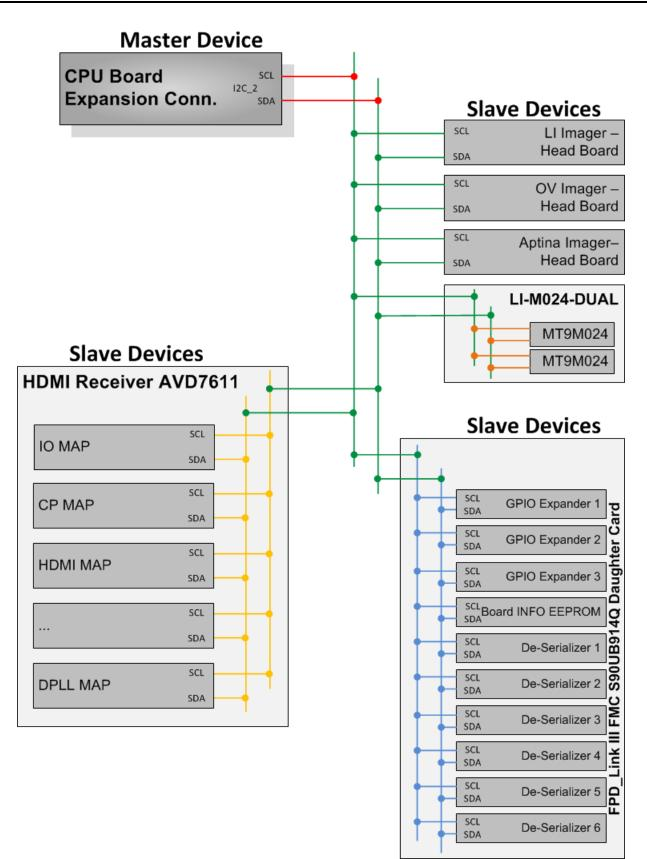
Figure 14. I2C Interface in Vision Apps Board
