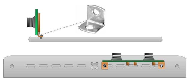
Figure 6. LI Dual Image Sensor Head Board Mounting
