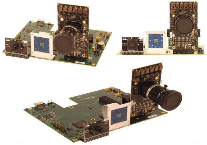
Figure 3. Board With Imager Head Board Stackup Views
