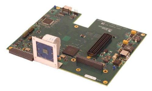
Figure 5. LI Image Sensor Head Board Assembly
