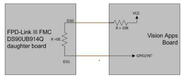
Figure 10. Board Presence Detection
