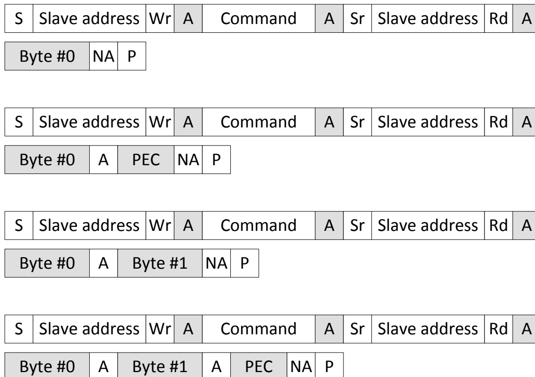
Figure 35-19. Read Byte and Read Word Messages With and Without PEC
