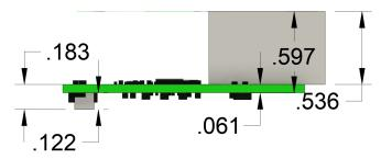
Figure 2-8. Industrial Ethernet PHY Add-on Board Side Profile
