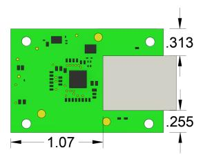
Figure 2-11. RJ45 Connector Position
