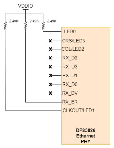
Figure 2-6. Industrial Ethernet PHY Strapping Resistors
