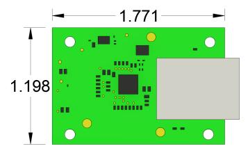
Figure 2-7. Industrial Ethernet PHY Add-on Board Dimensions
