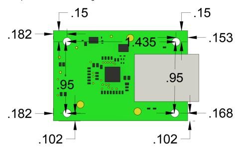
Figure 2-10. Mounting Hole Positions
