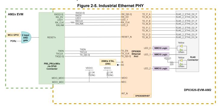
The Ethernet PHY requires two power sources, VDDIO (3.3V or 1.8V) and VDDA3V3 (3.3V) which are supplied through the DF40GB connector (J2).
