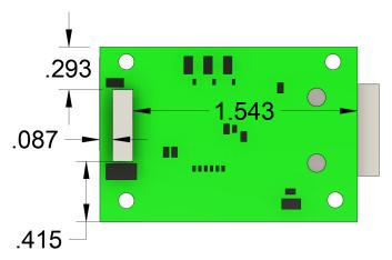
Figure 2-9. DF40GB Connector Mounting Position
