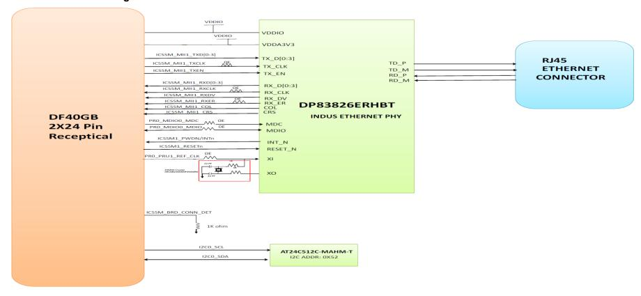
Figure 2-4. AM2x Industrial Ethernet PHY Add-on Board Block Diagram
