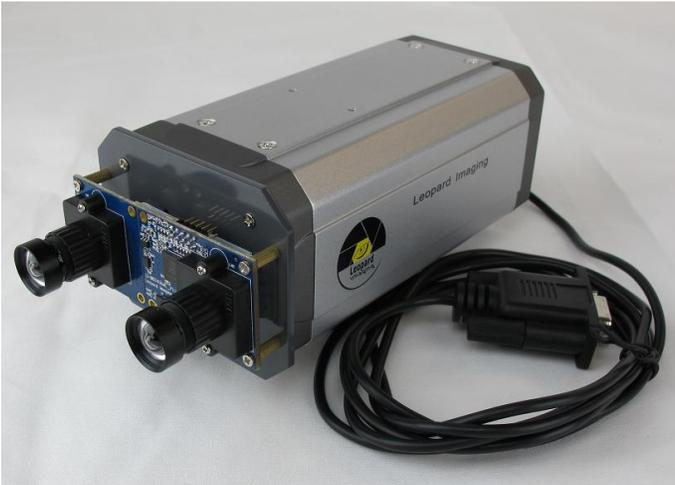
LNC-DUALCAM Module with serial cable
