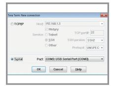
4 On the host computer, open a serial port terminal (like Tera Term or Hyperterminal for Windows® OS and minicom for Linux™ OS) and select the connection to the USB serial port.
