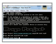
9 Once booting continues, the serial console will display additional start-up messages until a Linux login prompt is shown. At this point, Linux is up and running with a complete file system loaded from the SD card and you are ready to begin developing.
