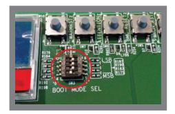
Set DIP switch (SW3) to '0111' (MSB first) as shown to select MMC/SD boot mode.
