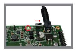
Connect 12V power cable to the DC jack (J3). Slide the power switch SW1 to the "ON" position marked on the silkscreen. LED LD9 will light up.
