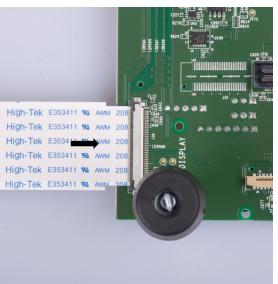
Note that if you need to pull the flex cable off, you can do so by simultaneously pressing on the connector metal strip and pulling the flex cable.
