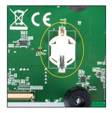
**Note:** This IDK is designed for optional use with a removable CR2032 UL recognized lithium battery (not supplied). Always use the CR2032VP Energizer 3V Lithium coin cell battery or similar CR2032 UL recognized battery with Nominal Voltage 3.0 Volts, Capacity 235mAh
