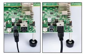
Connect the supplied USB debug cable to the USB connector labeled "UART" on the board. Connect the other end to your PC. Then open a serial console on your PC such as Teraterm. Please note that you may need to download and install an FTDI driver from
