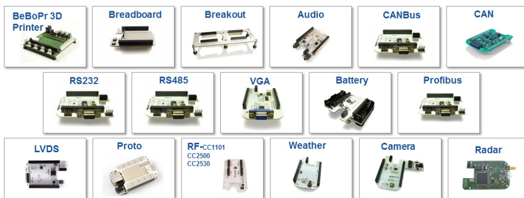
Figure 3. Cape plug-in boards easily expand the capabilities of BeagleBone Black.
