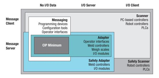
Figure 4. EtherNet/IP communications types and device classifications.
