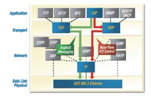
Figure 2. Multi-protocol support is possible because CIP is fully compatible with Ethernet and Internet protocols.
