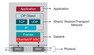
Figure 5. EtherNet/IP node.
