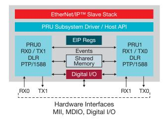
Figure 10. Firmware architecture.
