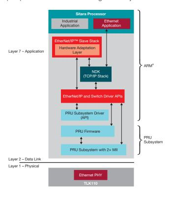
Figure 9. Software architecture for EtherNet/IP slave.
