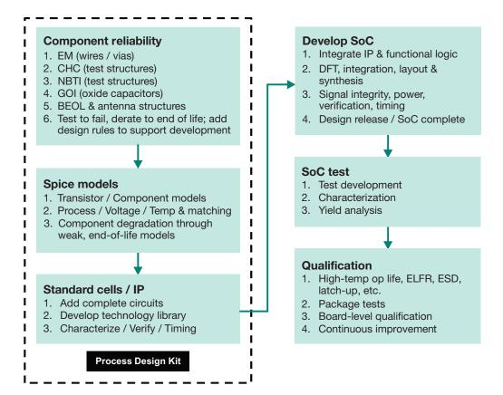
Figure 3: Design for intrinsic reliability process flow
