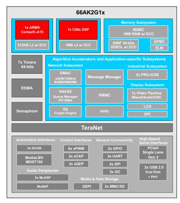
Figure 1: 66AK2Gx processor functional diagram
