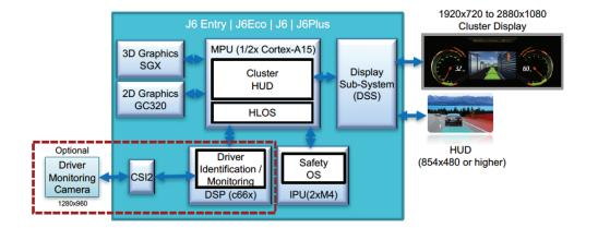
Figure 7. Jacinto 6 architecture to integrate driver monitoring and HUDs.
