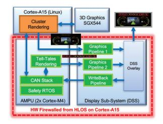
Figure 6. Jacinto 6 safety architecture based on AMPU.
