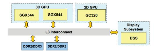
Figure 5. Jacinto 6 graphics and display subsystem architecture.
