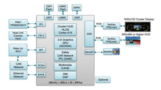
Figure 1. Digital cluster system block diagram.
