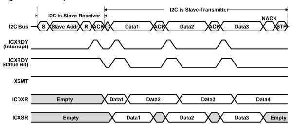
Figure 2. Interrupt Generation When XRDYM = 0
