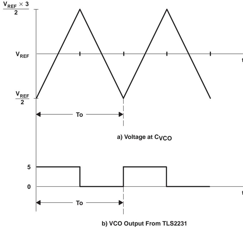
**Figure 9. VCO Waveforms**
