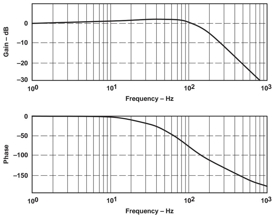
**Figure 11. Closed-Loop Frequency Response**
