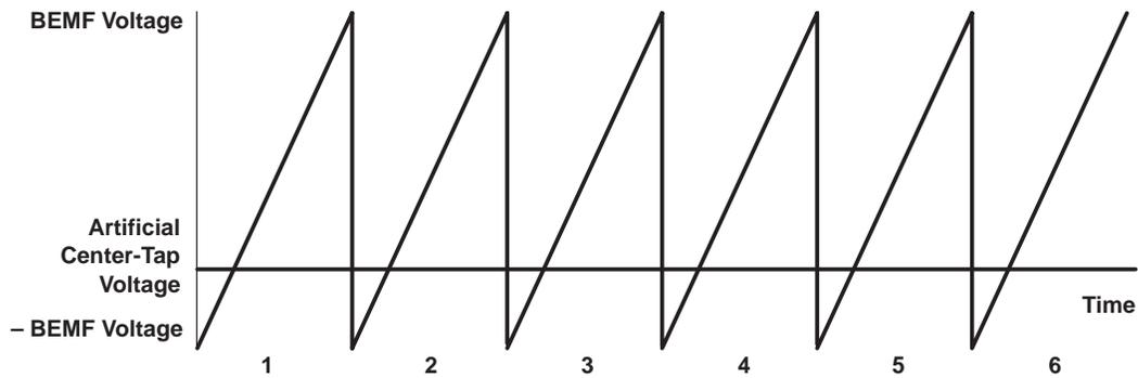
**Figure 7. Phase Comparator Waveform for Late Commutation**
