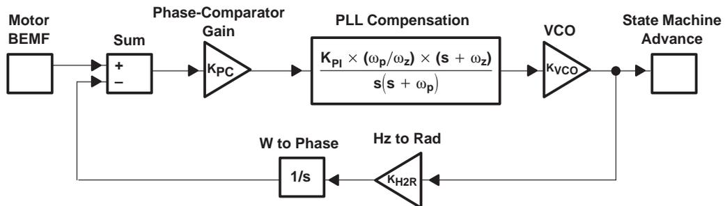
Figure 1. Matlab Model for TLS223x PLL
