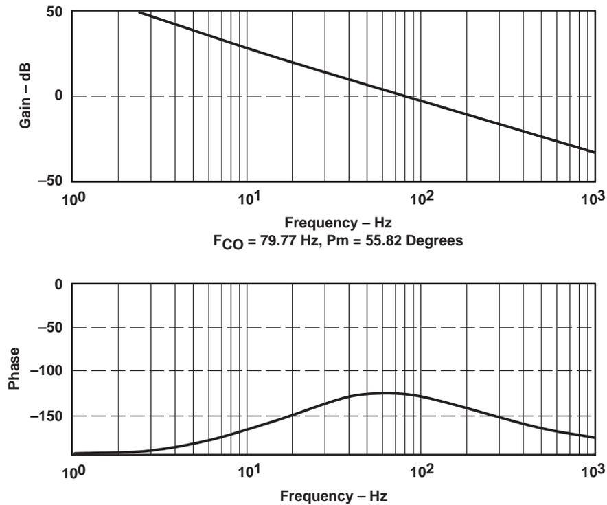
**Figure 10. Open-Loop Frequency Response**
