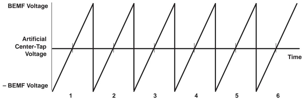
**Figure 6. Phase Comparator Waveform**
