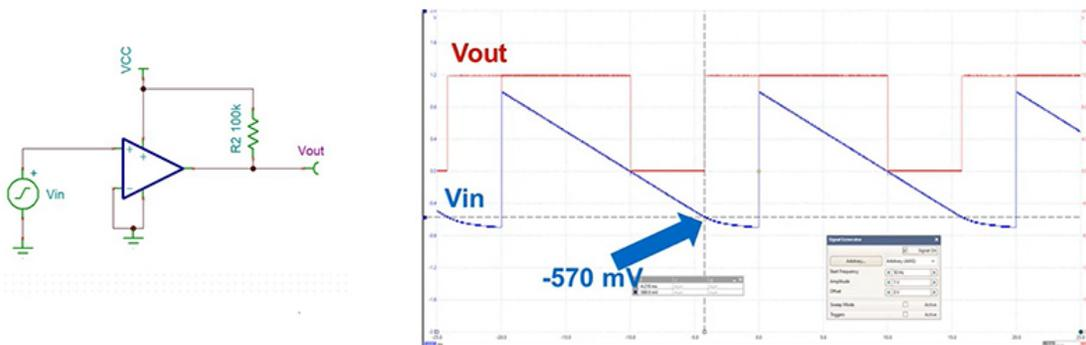
Figure 1. Phase Reversal in a Comparator
