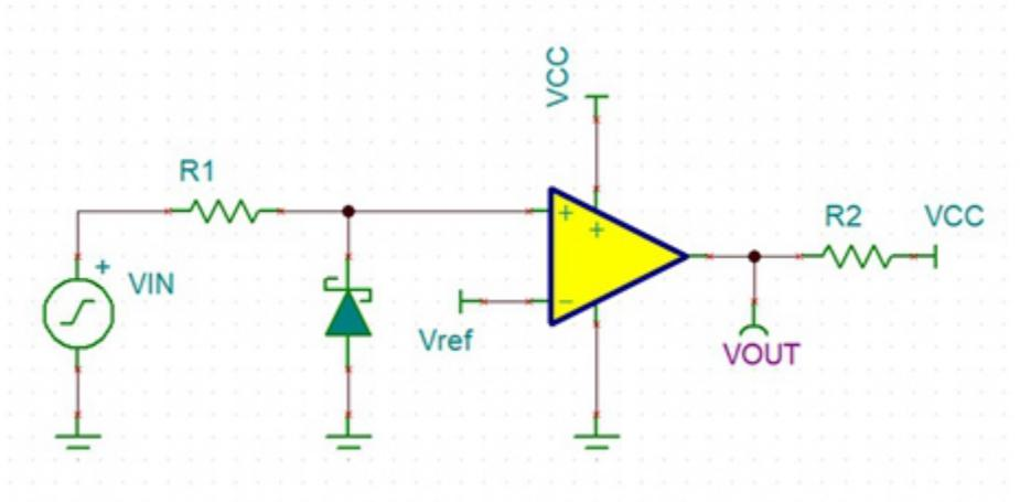
**Figure 3. Current-limiting Resistor with a Schottky Diode at the Input of the Comparator Circuit**
