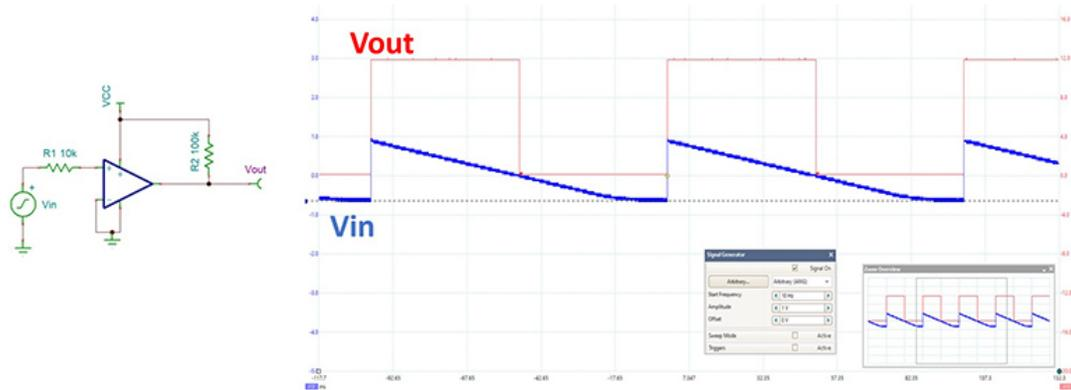
**Figure 4. The TLV1701'S Output Voltage with a Negative Input**
