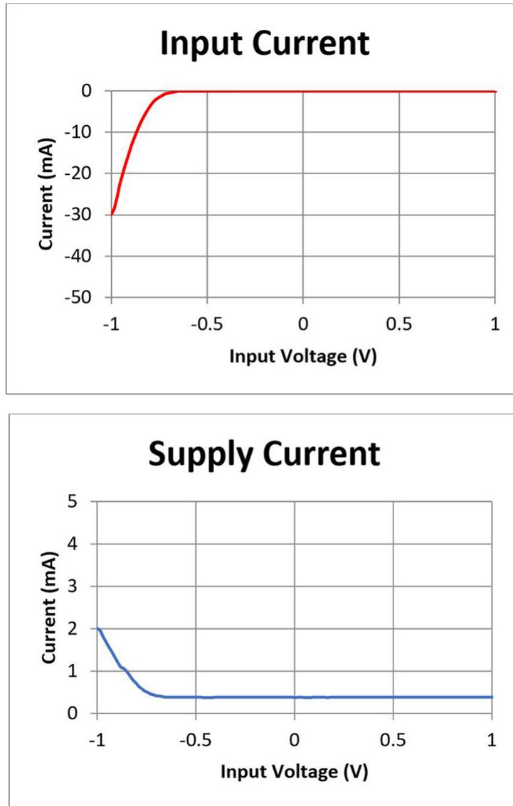
**Figure 2. Input Current and Supply Current Caused by Negative Input**
