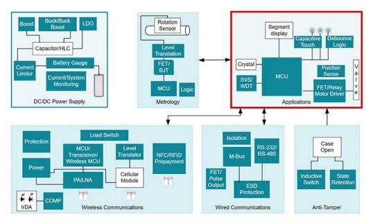
Figure 3. Reference Design for a Rotary Water Meter
