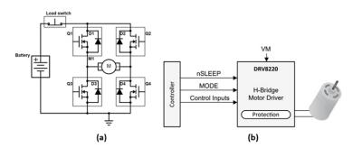
Figure 2. A Simplified Implementation of an H-bridge with Low-power Sleep Function Using an External Cut-off Switch (a); TI's DRV8210 with Automatic Sleep Mode (b)
