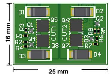
Figure 4. Discrete Implementation of an H-bridge and the Basic Surrounding Circuit; the PCB Area Is 16 Mm by 25 Mm, or 400 Mm<sup>2</sup>
