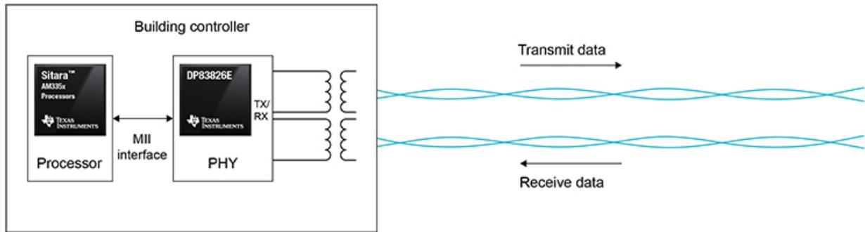
**Figure 2. Standard Ethernet Interface for 10/100-Mbps Communications in a Building Control Application**
