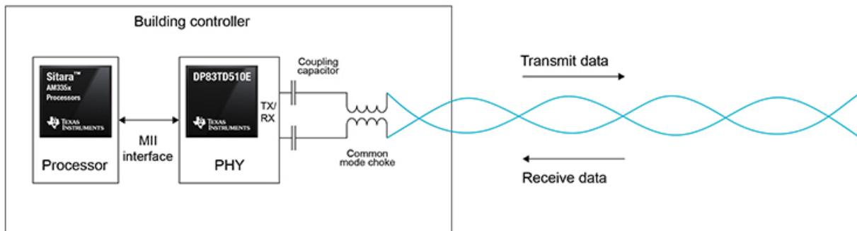
**Figure 3. Single-pair Ethernet Interface for 10-Mbps Communications in a Building Controller**
