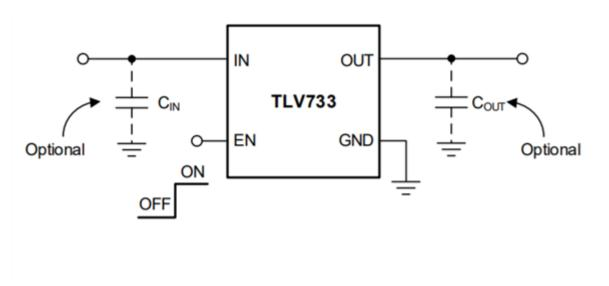
Figure 3. Simplified schematic diagram of the TLV33P
