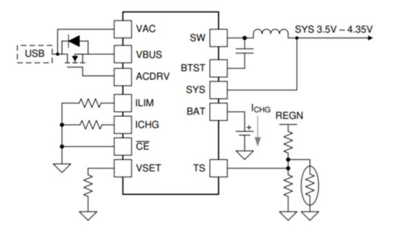
Figure 6. Simplified schematic diagram of the BQ25616
