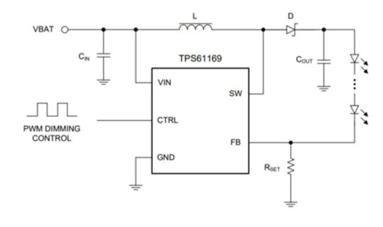
Figure 9. Simplified schematic diagram of the TPS61169
