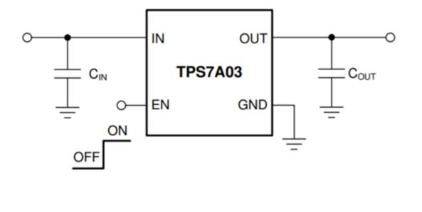
Figure 4. Simplified schematic diagram of the TPS7A03
