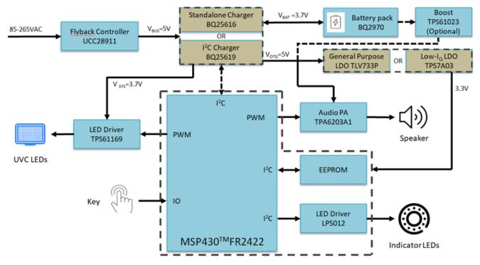
Figure 1. System block diagram of a UV sterilization box with a battery
