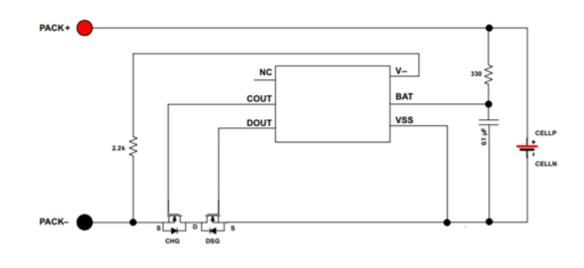
Figure 7. Simplified schematic diagram of the BQ2970
