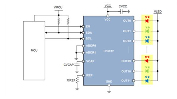
Figure 8. Simplified schematic diagram of the LP5012
