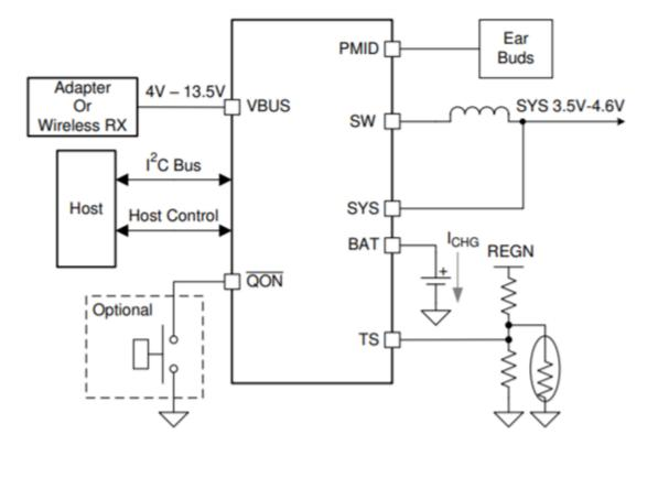
Figure 5. Simplified schematic diagram of the BQ25619
