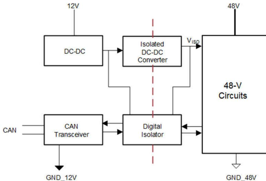
**Figure 2. Example of galvanic isolation between the 12-V and 48-V sides in a mild hybrid electric vehicle**
