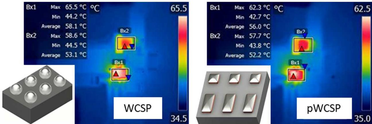
**Figure 2. Thermal performance of the TPS62088 (measurement point: Bx1) operating at  $V_{IN} = 5\text{ V}$ ,  $V_{OUT} = 1.8\text{ V}$  and  $I_{OUT} = 3\text{ A}$  taken at room temperature: TPS62088YFP WCSP version (a); TPS62088YWC power WCSP version (b)**
