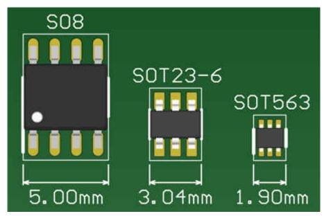
Figure 1. Mechanical outline sizes of three converter packages
