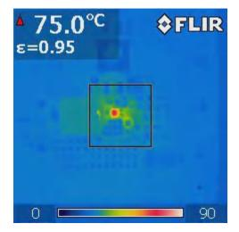
Figure 4. Thermal image of the TPS562231 with a 12-V input voltage
