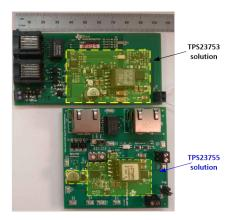
Figure 1. Board Space Comparison for TPS23755 vs. TPS23753
