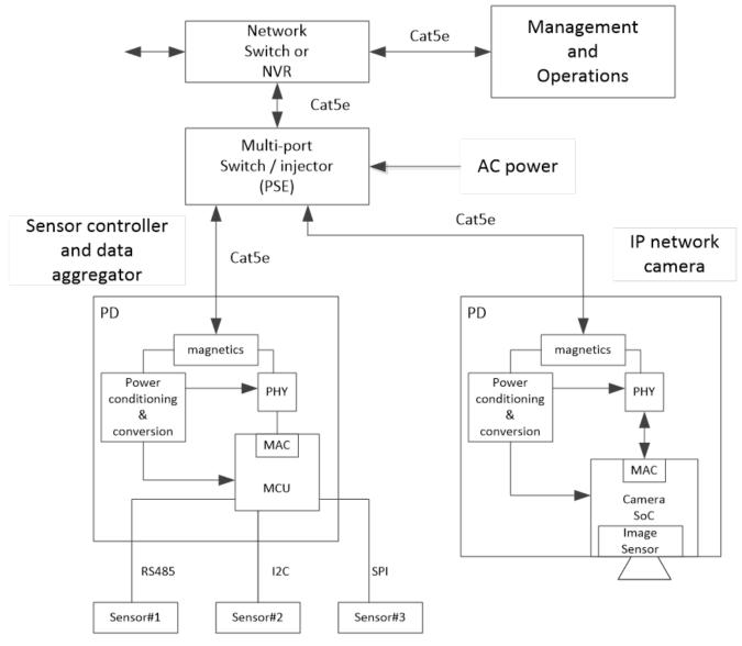
Figure 1. Example of a Building Automation Network Topology
