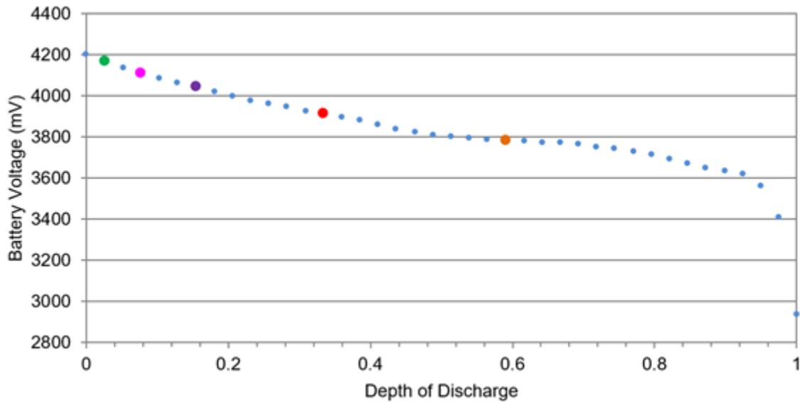
**Figure 2. Li-ion DOD versus Battery Voltage**
