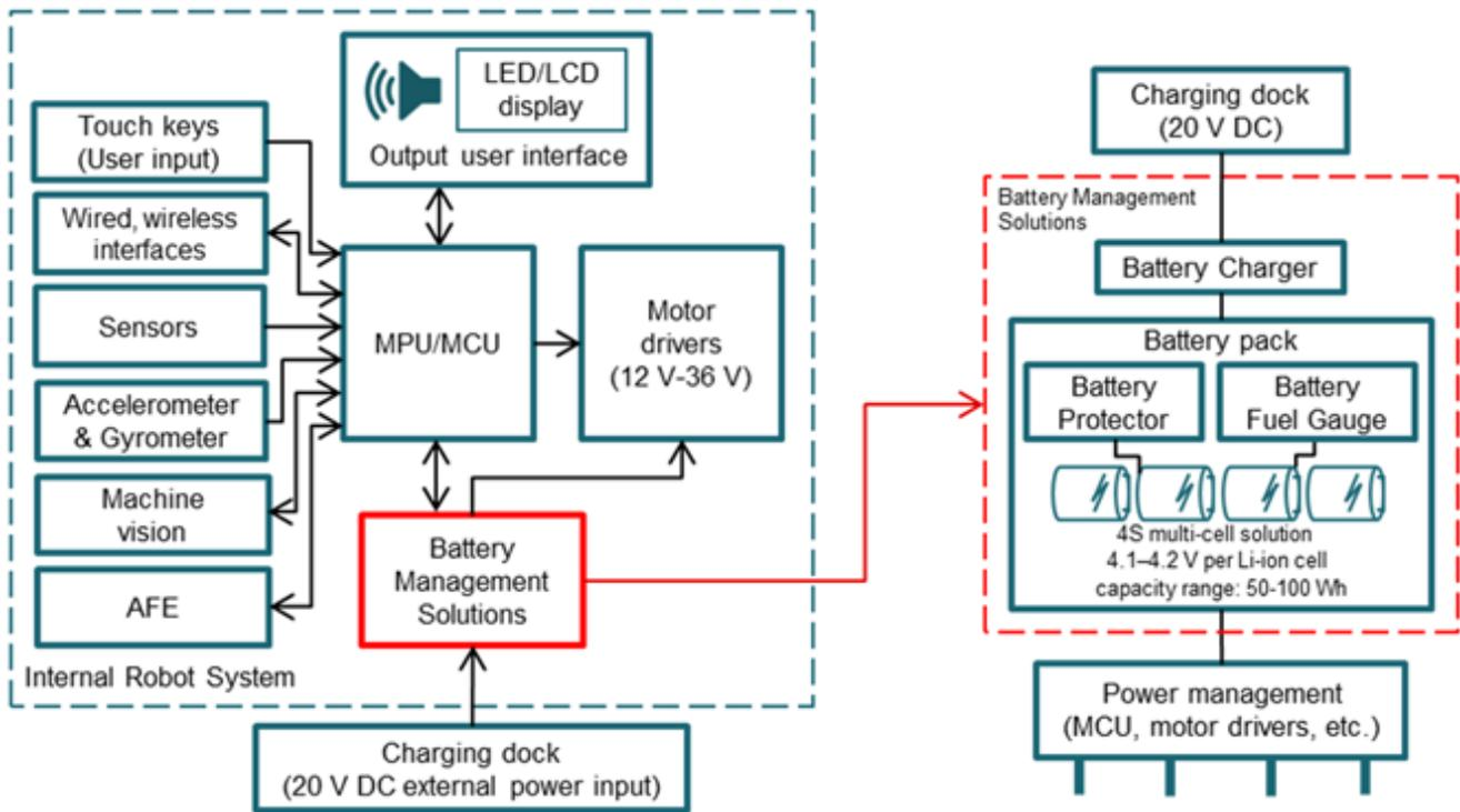
**Figure 1. Vacuum Robot System Power Diagrams**
