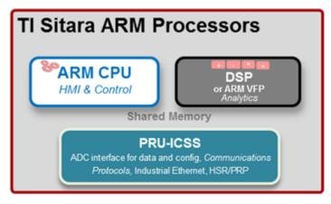
Figure 1. Overview of Sitara Processor with Arm Cores
