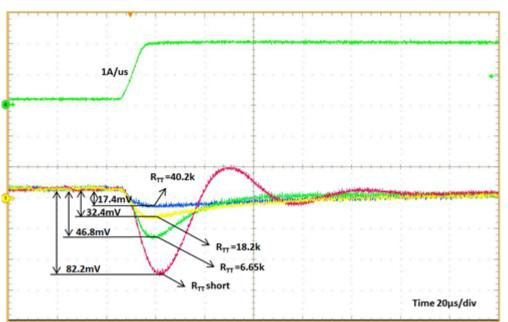
Figure 5. Transient Response with TurboTrans Technology
