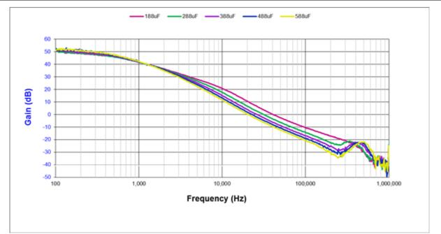
Figure 3. Gain Curve with Different Output Capacitance
