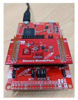
Figure 2. MSP-EXP432P401R LaunchPad Development Kit and BOOSTXL-SENSORS BoosterPack Module with SimpleLink SDK Plug-in Support
