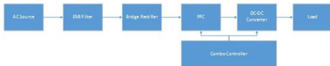
**Figure 2. Combo Controller IC-based AC/DC Design**
