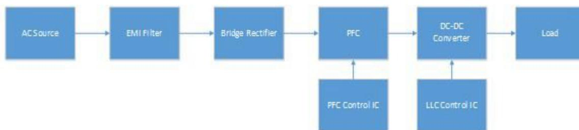
**Figure 1. Discrete Controller IC-based AC/DC Design**
