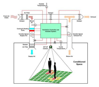
Figure 1. 3D ToF Camera-based DCV System
