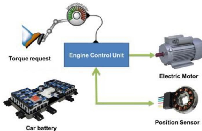
Figure 1. Typical System Block Diagram of a Motor-control System in a Vehicle
