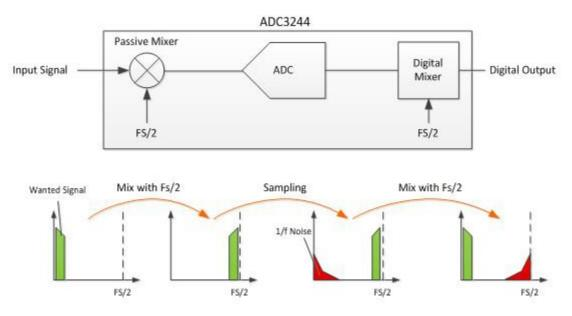
Figure 2. Chopper Implementation Details of the ADC3244
