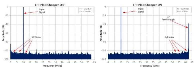
Figure 3. A 10MHz Input Signal with the Chopper Disabled (Left) and Enabled (Right)
