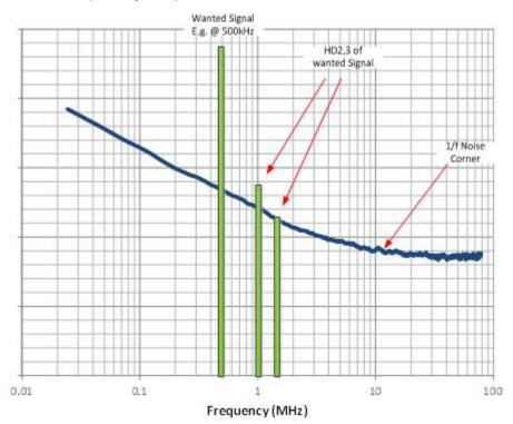
Figure 1. Wanted Signal and Its Harmonics in the Presence of 1/F Noise
