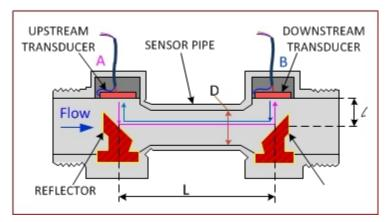
Figure 1. Ultrasonic Sensor Cell
