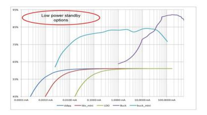
Figure 2. The TPS65290'S Efficiency Curve of Various Blocks Can Significantly Improve System Efficiency
