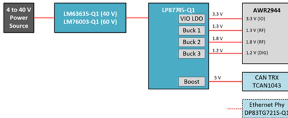
**Figure 1. The LP87745-Q1 powering the AWR2944 radar chip for corner radar applications**
