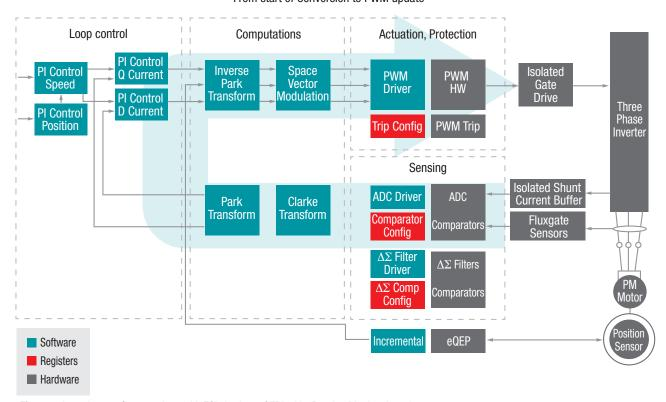
Figure 1. Less than 1 uS current loop with FCL (replace "QEP" with "Resolver" in the picture).
