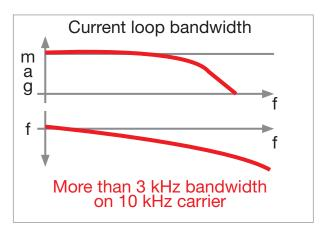
Figure 2. Improving current loop bandwidth while maintain carrier frequency.
