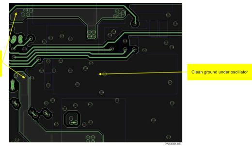
Noisy ground (DCDC ground) not connected to reference or oscillator ground
