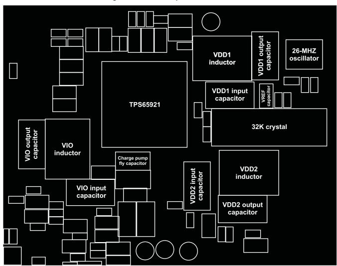
**Figure 1. Critical Component Placement**
