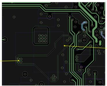
Dedicated ground shape connecting VIO.GND, input capacitor ground, and output capacitor ground only
