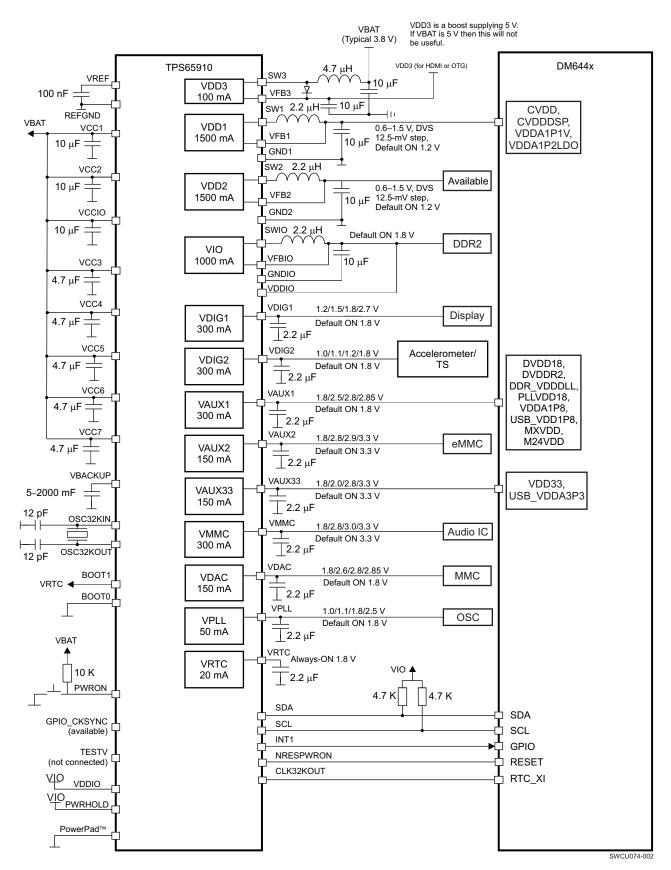
Figure 2. DM644x Power Supply Connections With TPS659105
