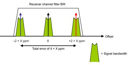
Figure 1. Plot of IF Versus Frequency Error
