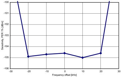
Figure 5. 4.8 kbps, MDMCFG2.DEM\_DCFILT\_OFF = 1
