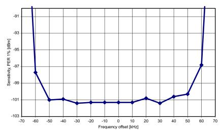
Figure 8. 38.4 kbps, MDMCFG2.DEM\_DCFILT\_OFF = 0
