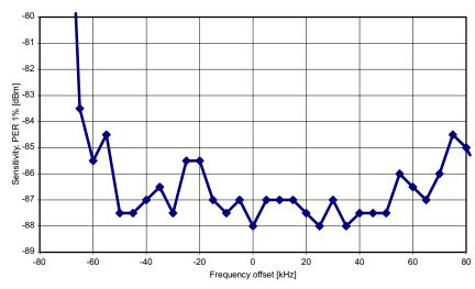
Figure 12. 500 kbps, MDMCFG2.DEM\_DCFILT\_OFF = 0
