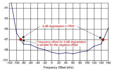
Figure 2. Definition of Frequency Offset That Gives 3-dB Degradation on PER (Unsymmetrical Frequency Offset)
