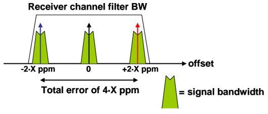
Figure 1. Plot of IF versus Frequency Error
