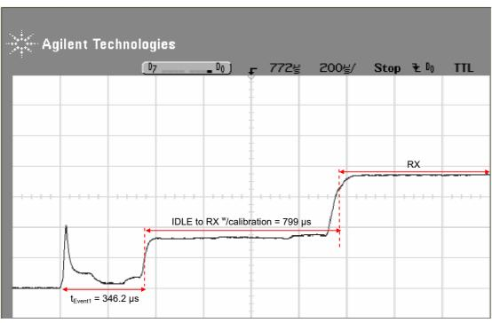
Figure 3. Current Consumption Test Case 1 (start-up sequence)
