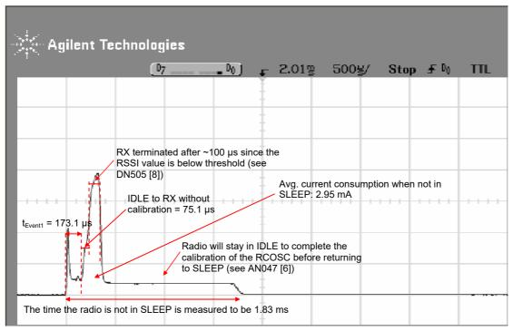
Figure 20. Current Consumption Test Case 6
