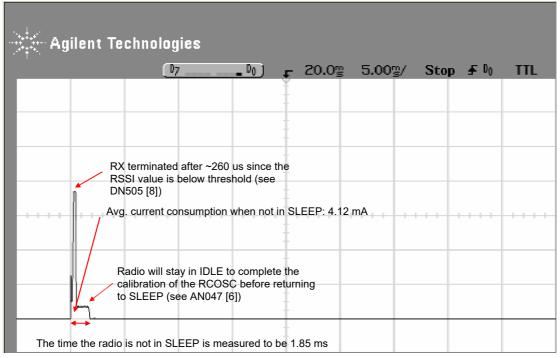
Figure 8. Current Consumption Test Case 3
