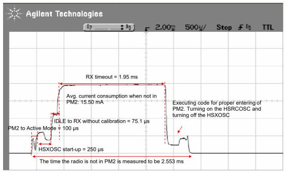
Figure 36. Current Consumption Test Case 11
