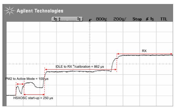
Figure 28. Current Consumption Test Case 7 (start-up sequence)
