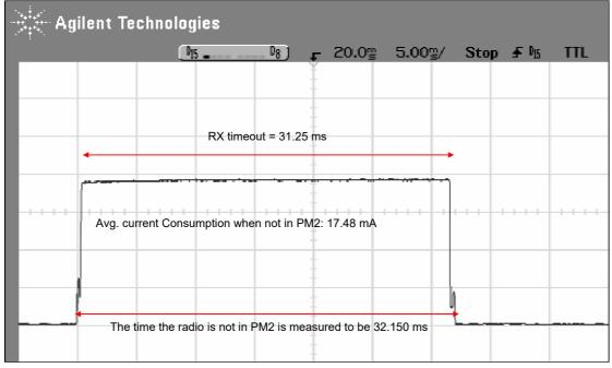
Figure 29. Current Consumption Test Case 8
