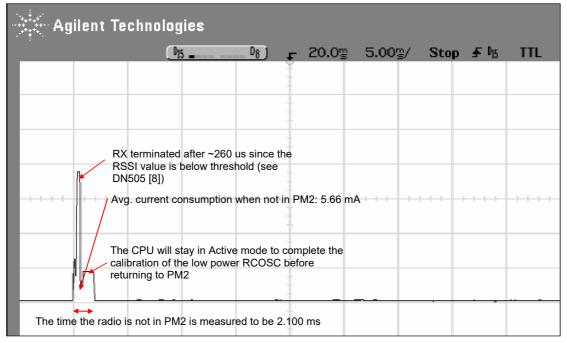
Figure 31. Current Consumption Test Case 9
