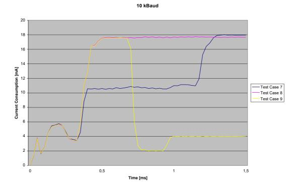
Figure 34. Test Case 7 - 9 (start-up sequence)
