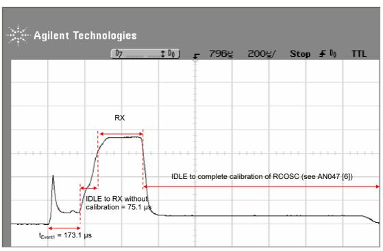
Figure 9. Current Consumption Test Case 3 (start-up sequence)
