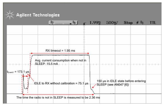
Figure 17. Current Consumption Test Case 5
