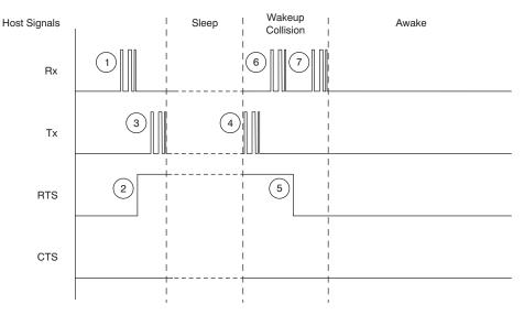
Figure 5. Wake-Up Collision Type 2
