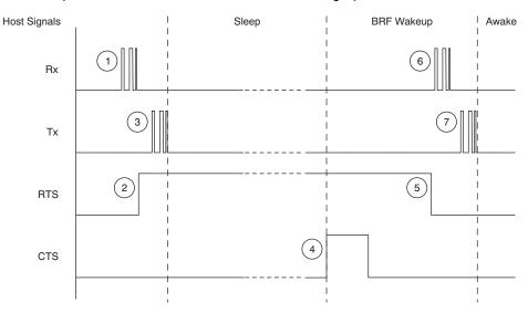
Figure 2. Wake-Up by Baseband Controller
