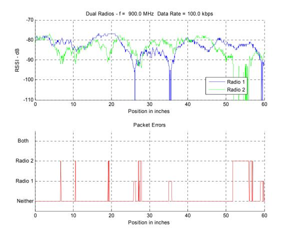
Figure 12 - Dual Radios, 900 MHz, 100 kbps
