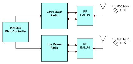
Figure 4 - Dual Radio Two Antenna Diversity
