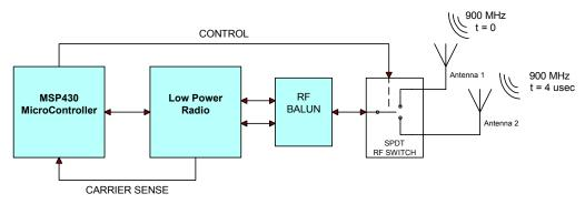
Figure 2 - Single Radio Amplitude-Based Antenna Diversity
